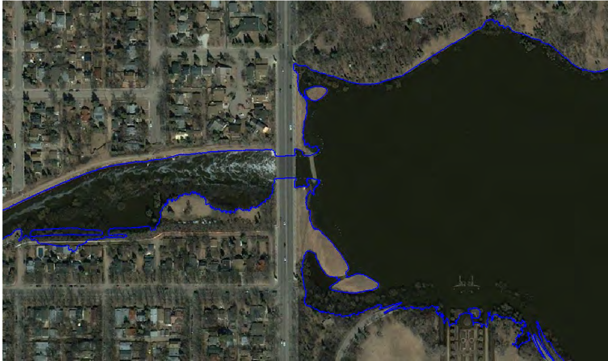
Figure 5-5: Simulated Flood Inundation in Wascana Creek at Albert St. (Blue Line) Against Observed Flood Extension on April 26, 2011 (Aerial Photo)
