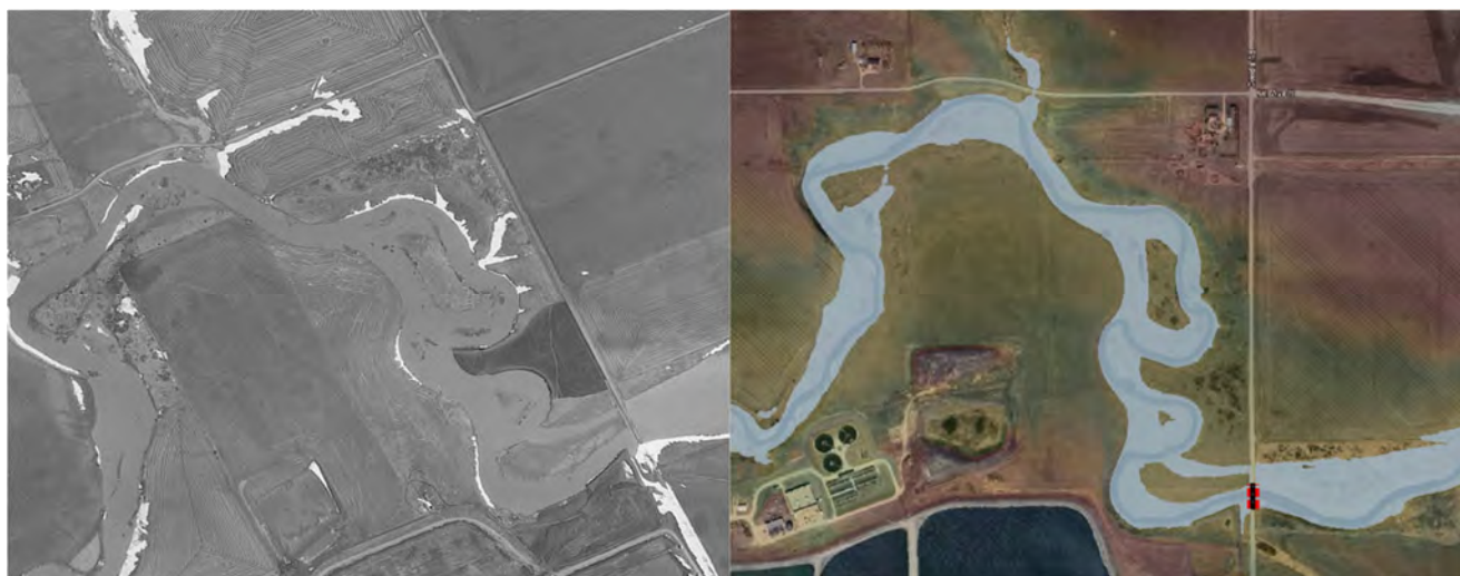
Figure 5-9: Simulated Flood Inundation in Wascana Creek at Lagoons (Right) Against Observed Flood Extension on April 22, 1974 (Left)
